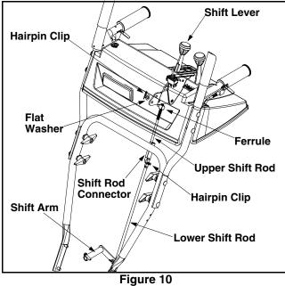
Reconnect the upper shift rod to the lower shift rod by reinserting the hairpin clip removed earlier and sliding the shift rod connector back down into place.
